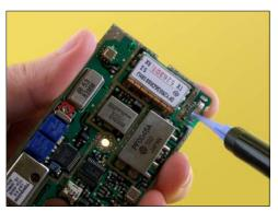
Master Bond's electrically conductive adhesives, sealants and coatings are widely used in the electronic and electrical industries. They are formulated with metal powders and flakes such as silver, nickel, copper and silver-coated nickel, with silver formulations exhibiting the highest levels of electrical conductivity. Graphite filled formulations have also been developed for use where metal additives are not desirable. Master Bond offers a number of room temperature curing
